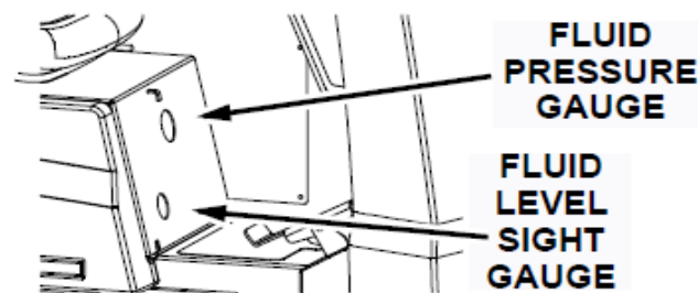
Fig. 3: Hydraulic Fluid Gauges
